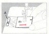
· Lift right edge of slide plate and draw it to the right until it is disengaged from spring A.
