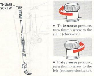
Adjustment of the thumb screw regulates the amount of pressure exerted on the material while it is being stitched.
