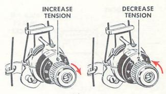
• To increase tension, turn the thumb nut to the right (clockwise) until required tension is obtained Each higher number denotes increased tension.  To decrease tension, turn the thumb nut to the left (counter-clockwise) until the required tension is obtained. Each lower number denotes less tension.
