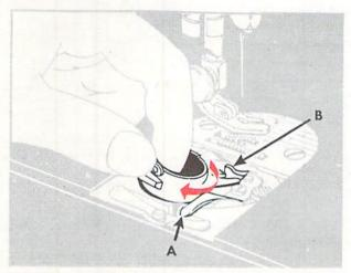
To clean stitch forming mechanism, remove bobbin case as follows—
