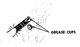
Motor for gear drive with grease cups. Machines 201 and 15-91.
