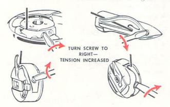
When the tension on the bobbin thread has been properly adjusted, it is seldom necessary to change it, as a correct stitch can usually be obtained by varying the tension on the needle thread.
